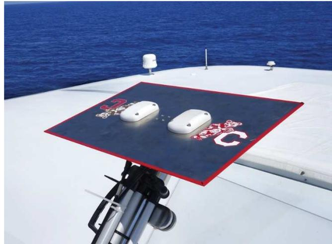
**Fig 1.** A GPS spoofing-detection system above the bridge of the supervacht. Photo: Mark L. Psiaki
