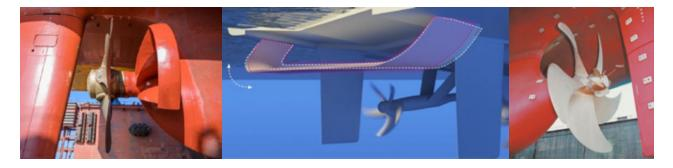
ESDs come in many types and forms. Fins, spoilers, wedges and interceptors reduce the wave-making losses and typically apply to ships sailing a high-speed range. Ducts and pre-swirl stators optimize propulsion losses. Post-swirl devices and optimized rudders reduce or recover part of the energy losses due to the propeller action.
