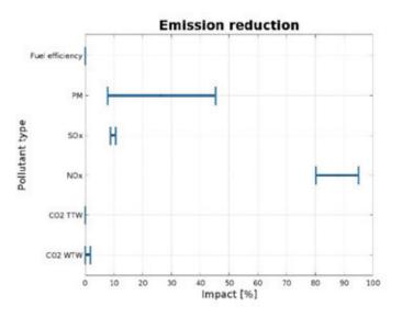
GHG & pollutant reductions when using a SCR aftertreatment installation.
